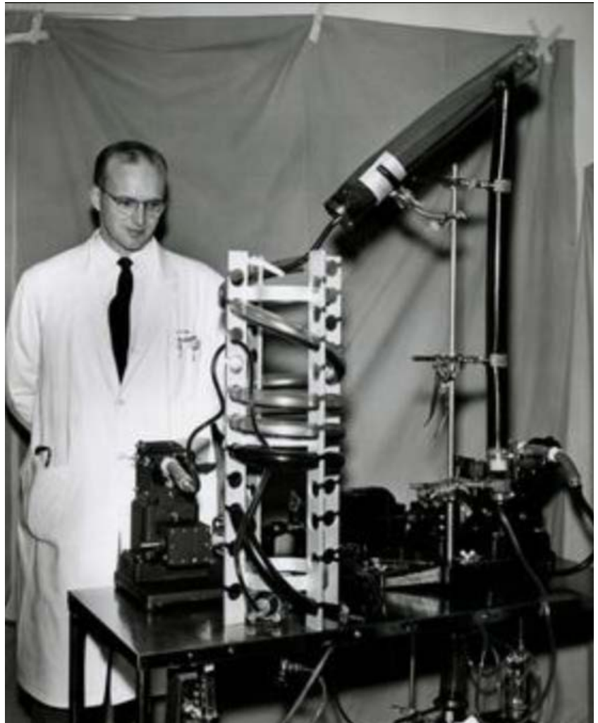
The helical reservoir bubble oxygenator, invented by Richard DeWall (pictured) and C. Walton Lillehei, made open-heart surgery a practical procedure. Courtesy University Archives. Minnesota Research Firsts in Medical Devices, Procedures, Health Care, and Bioscience. https://mbbnet.ahc.umn.edu/firsts/historic.html , accessed Jan. 16, 2024
